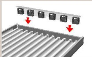
Stealth's extraordinary performances are enhanced in the version provided with Cooling System. These models have adjustable speed fans, that change referring to the internal temperature.
